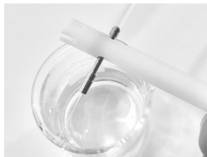
Figure 26: Flushing the microvalve.
