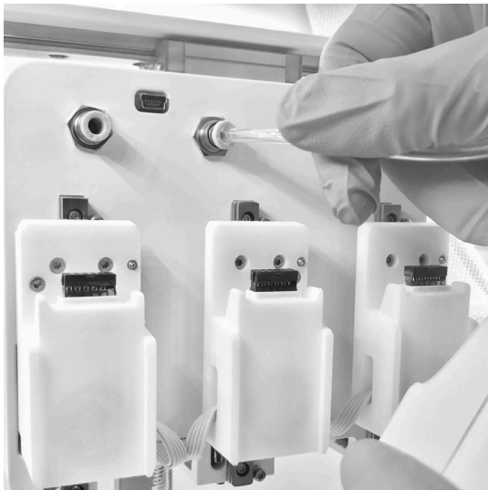
Figure 12: Attaching the EMD Printhead to the BIO X printhead mount.
