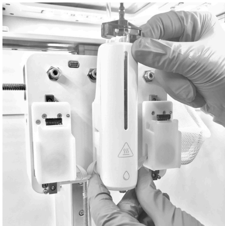
Figure 4: Inserting the EMD Pneumatic Printhead into the BIO X system.
