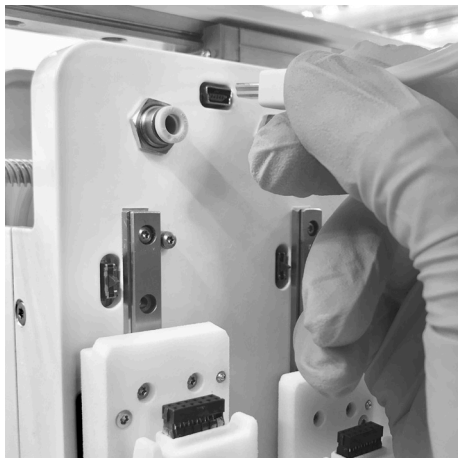
Figure 4: Attaching the micro-USB to the BIO X printbox.
