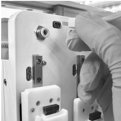
Figure 10: Detaching the micro-USB from the BIO X.
